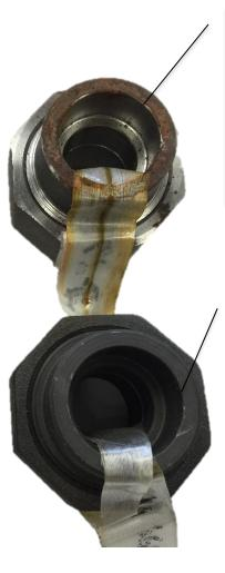
Rust Noticed on Face of fittings as well as other areas of fittings that were Oil Coated, It is evident that the oil is not systematically applied, leaving areas un-protected.
