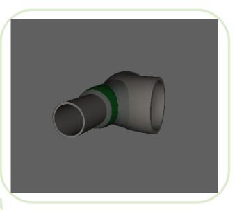
Equation for overall length L = E + $\sqrt{B^2-A^2}$  + Root gap
